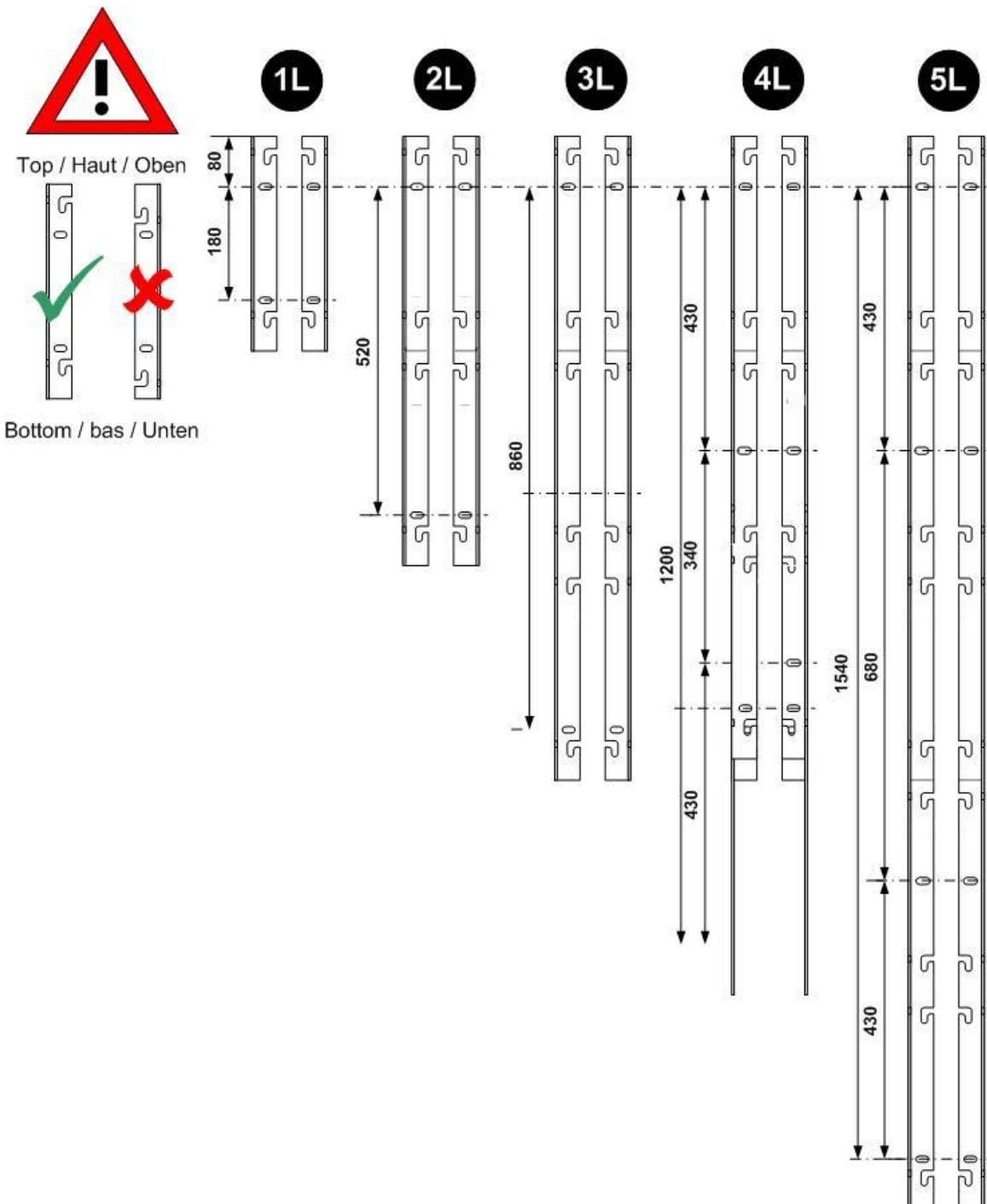
It is possible to mount the brackets so that they are «HIDDEN» or «VISIBLE». Use the corresponding drilling measurement according to the chosen mounting method.
