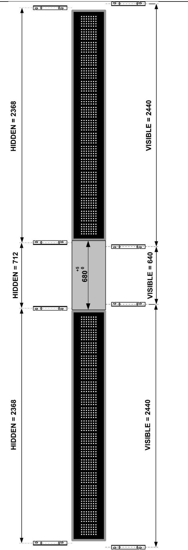
Before mounting the Calypsos on their support, mount the 4 screws M8x20, as in the drawing below, without tightening them. First mount the board situated on the bottom of the column by using the hooks of the brackets. Do the same with the upper line and so on until the top of the column.
