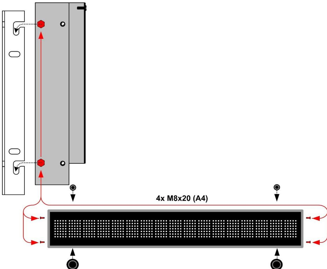
Once all the lines are mounted, slightly tighten the M8x20 screws. On the upper line, mount the small Ø caps, and on the lower line, mount the big Ø caps.
