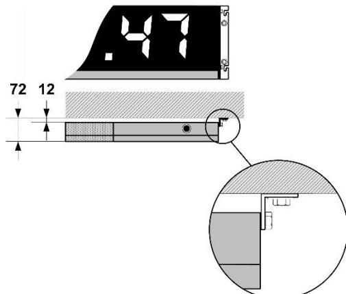
The mounting kit contains the plugs for fixing into a concrete wall (CONCRETE) or the screws for a metallic support (METALLIC).
