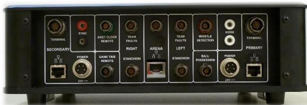
Figure 4 - Connection panel of the FSTT
