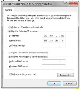
Note: IP address is 192.168.2.100 for OSV MYRIA connection and 192.168.0.100 for OSV-STAR connection.
