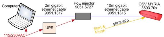
Connect the 10m network cable Ethernet Gigabit (9051.1315) between the Ethernet connector on the camera and the PoE connector of the PoE injector (power supply). Connect the 2m network cable Ethernet Gigabit (9051.1317) between the LAN connector of the PoE injector and the computer.
