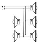
5 Speakers of 16 Ohms each Total load of 3.2 Ohms
