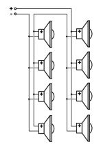
8 Speakers of 16 (8) Ohms each Total load of 8 (4) Ohms
