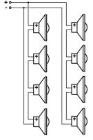
8 Speakers of 4 (8) Ohms each Total load of 8 (16) Ohms
