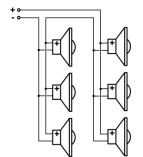
6 Speakers of 16 (8) Ohms each Total load of 10.6 (5.3) Ohms
