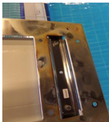
OSB poorly maintained
