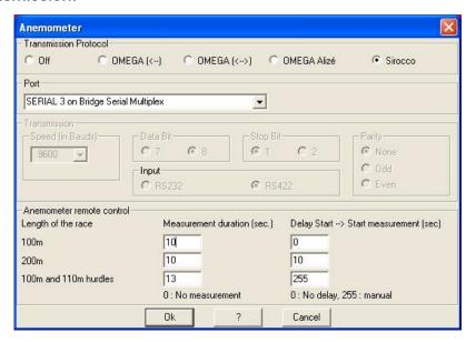
Then select the port ("SERIAL 3 on Bridge Serial Multiplex" or "SERIAL 4 on Bridge Serial Multiplex") according to the hardware connection you made.
