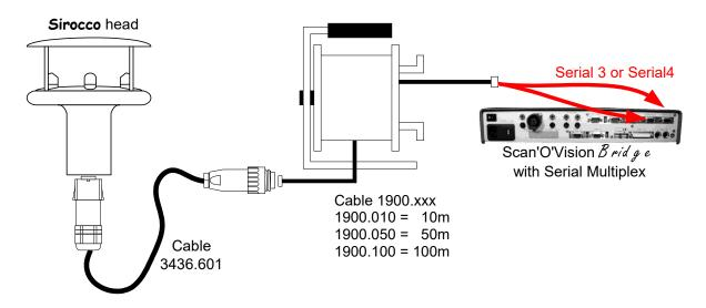
Optional extended cable can be plugged between the cables 3436.601 and 1900. series cable (up to 400 meters).
