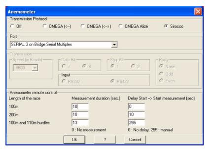
Then select the port ("SERIAL 3 on Bridge Serial Multiplex" or "SERIAL 4 on Bridge Serial Multiplex") according to the hardware connection you made.
