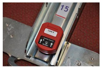
Fixing clips are permanently fixed on starting blocks. MoSen is then easily mounted, dismounted on the clip without any tool.
