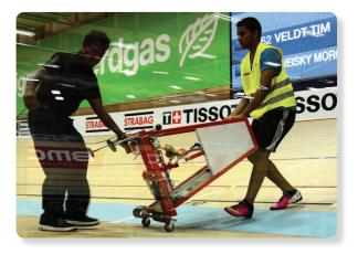
On one side, two rubber bases keep the contact with the track floor when the gate is installed. The bases are complemented by two wheels, allowing quick and easy removal from the racing track.
