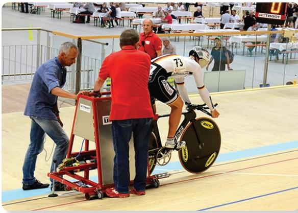
The stability of the starting gate allows the athlete to await the start signal whilst seated on the cycle, allowing the athlete to concentrate on the race start.
